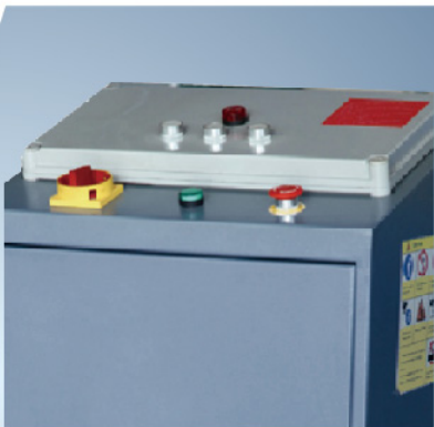
Low Voltage Control Unit
